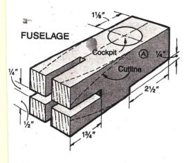
And with a bandsaw or a dado blade mounted in your radial-arm or tablesaw, cut the rabbet in the underside of the fuselage.
