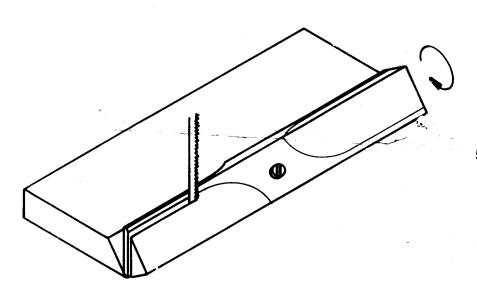
5. Remove the Wood Screw, turn the Whirlygig Wing over, reattach the Screw, and repeat Steps 3 and 4.
