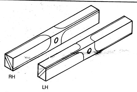
2. Layout the Whirlygig Wings on 3/4" x 1" x 8" blocks (1 LH & 1 RH REQ'D) and drill the 3/16" Dia. hole through.
