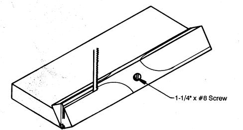
3. Mount the Whirlygig Wing to the bevel with a 1-1/4" x #8 Round Head Wood Screw. Make the first cut on a bandsaw with a 1/8" blade.
