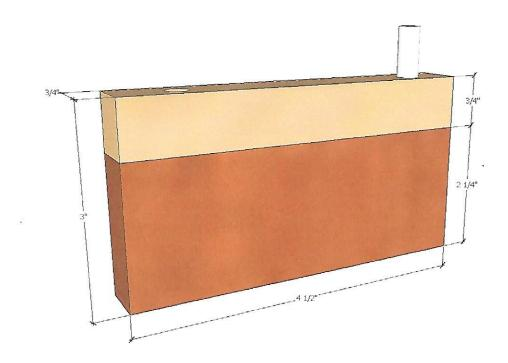
The camera is made from contrasting woods. The UPPER piece is usually lighter color than the LOWER piece. It is very important you make the width of UPPER and LOWER exactly the same or the operation of the camera will be compromised.
